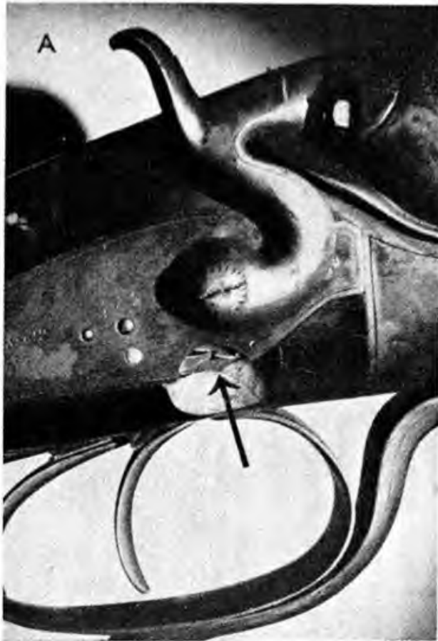
(A) THE RIGHT LOCK OF THE GUN IN PLATE XI IN THE REBOUND POSITION All the parts of the lock are properly adjusted and the sear nose is right up in the bent (see arrow)
