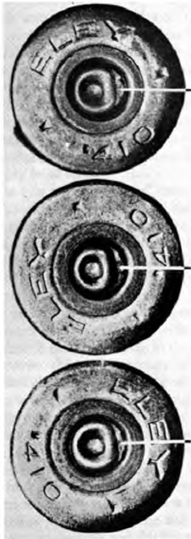
THREE DIFFERENT .410 SHOTGUN CARTRIDGE CASES ALL OF WHICH WERE FIRED BY THE SAME GUN
