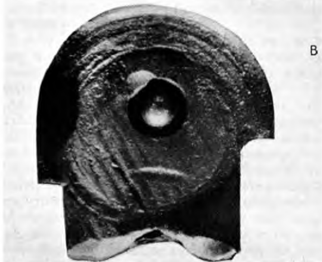
(A) THE BREECH FACE OF A HIGH-GRADE, HAND-FINISHED REVOLVER (B) THE BREECH FACE OF A MACHINE-FINISHED SELF-LOADING PISTOL
