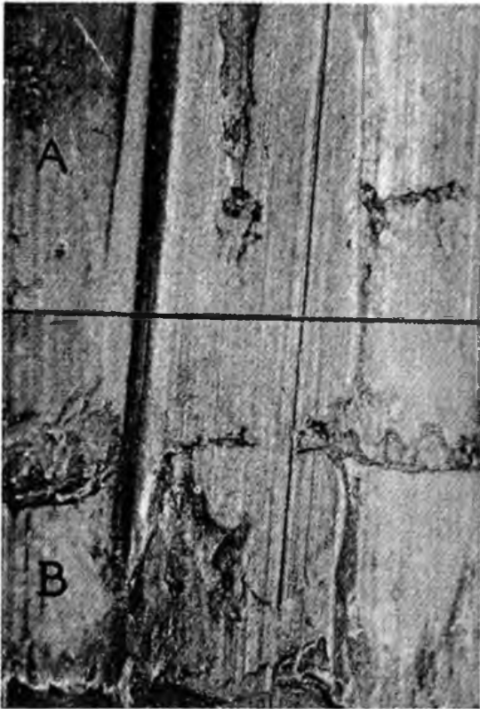
COMPOSITE PHOTOGRAPHS SHOWING HOW THE MARKINGS ON BULLETS FIRED BY THE SAME WEAPON MATCH EXACTLY A and B are the two bullets shown in Plate XXXI. In this Plate the upper part of the left-hand photograph is A, while the lower part is B; and in the right-hand photograph the upper part is B, while the lower is A. In both photographs the striations match exactly
