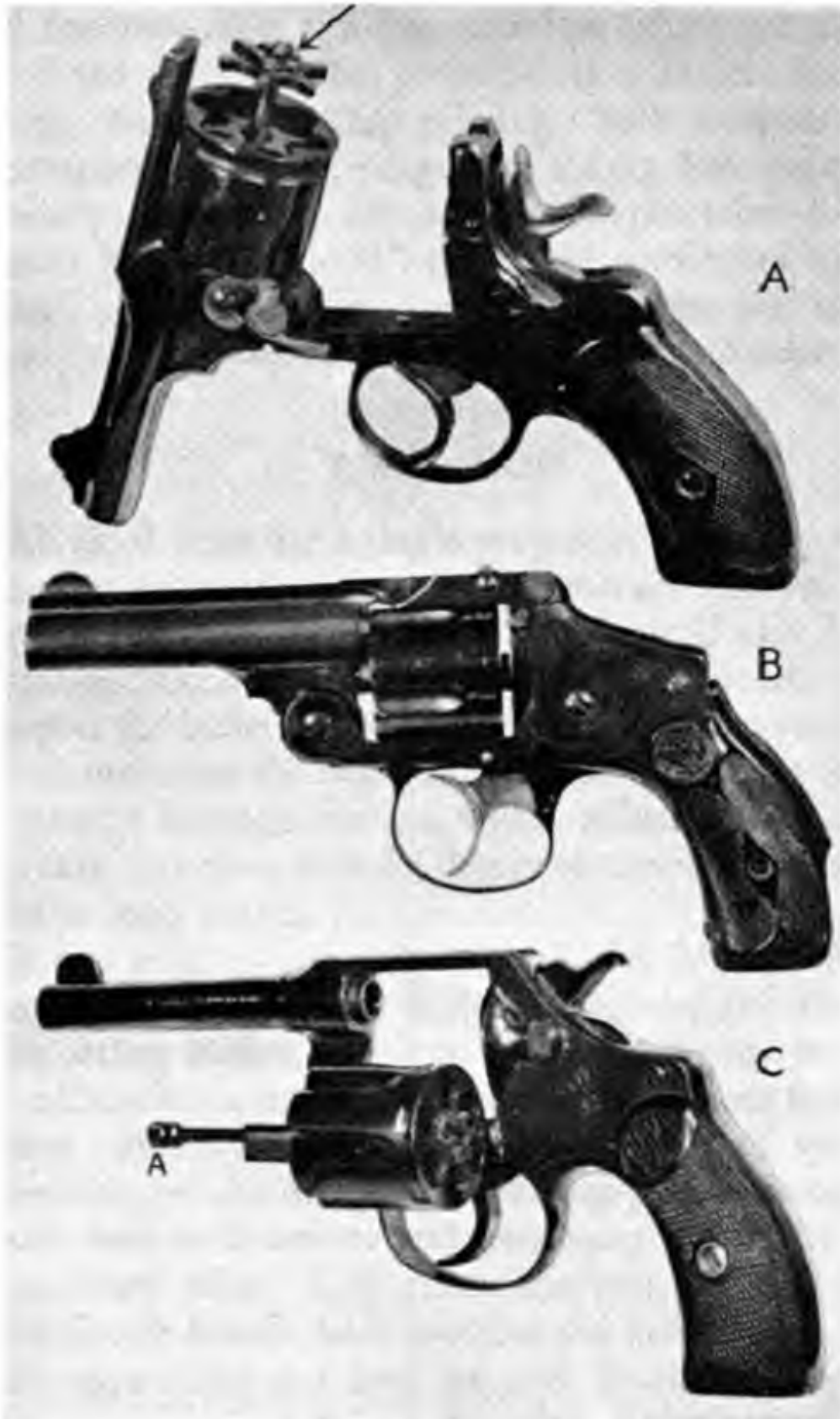
(A) A WEBLEY "BREAK DOWN" MODEL REVOLVER OPEN AFTER FIRING The arrow indicates the extractor (B) A SMITH AND WESSON HAMMERLESS "BREAK DOWN" MODEL REVOLVER (C) A COLT "SOLID FRAME" MODEL REVOLVER OPEN READY FOR LOADING Extraction is effected by pushing to the rear the rod indicated by letter A
